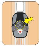
Hold the sensor button until the monitor beeps three times.
