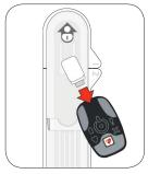
Remove patch from packaging. Connect cable to monitor.
